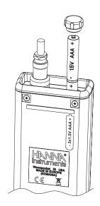
The instrument is provided with the BEPS (Battery Error Prevention System) feature, which automatically turns the instrument off when the batteries level is too low to ensure reliable readings. At start up the display will show "0 bAtt" message for a few seconds, then the instrument automatically turns off.
