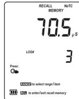
Press **Range** and the instrument will display the next logged parameter as shown in the table below:
