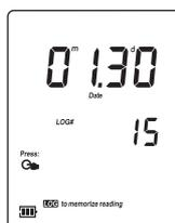
The instrument will display the current date (mm.dd) on the primary LCD, the record number on the secondary LCD and then the number of available tags remaining.
