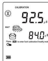
Select the desired calibration value with the ARROW keys, if necessary.
