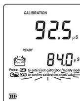
Press **CFM** (or **2nd** then **CFM**) to confirm calibration.
