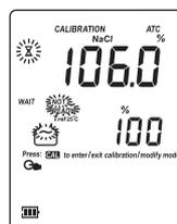
When the reading is stable, the “**READY**” tag will be displayed and the “**CFM**” tag starts blinking on the LCD, asking for confirmation.
