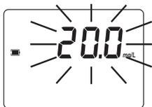
**Over Range:** A flashing value of the maximum concentration indicates an over range condition. The concentration of the sample is beyond the programmed range: dilute the sample and re-run the test.
