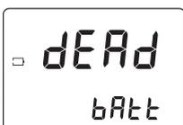
**Dead battery:** This indicates that the battery is dead and must be replaced. Once this indication is displayed, the meter will lock up. Change the battery and restart the meter.
