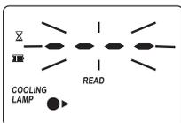
**Cooling lamp:** The instrument waits for the lamp to cool down.
