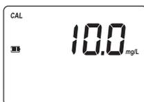
*Note: If the display shows "STD HIGH", the standard value was too high. If the display shows "STD LOW", the standard value was too low. Verify that both CAL Check™ Standards HI96709-11 Cuvettes, A and B are free from fingerprints or dirt and that they are inserted correctly.*
