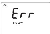
**Standard Low:** The standard reading is less than expected.
