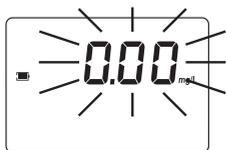
**Under range:** A blinking "0.00" indicates that the sample absorbs less light than the zero reference. Check the procedure and make sure you use the same cuvette for reference (zero) and measurement.
