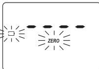
**Battery low:** The battery must be replaced soon.
