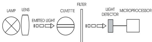
A microprocessor controlled special tungsten lamp emits radiation which is first optically conditioned and beamed to the sample contained in the cuvette. The optical path is fixed by the diameter of the cuvette. Then the light is spectrally filtered to a narrow spectral bandwidth, to obtain a light beam of intensity  $I_0$  or  $I$ .
