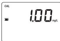
*Note: If the display shows “STD HIGH”, the standard value was too high. If the display shows “STD LOW”, the standard value was too low. Verify that both CAL Check™ Standards HI96701-11 Cuvettes A and B are free of fingerprints or dirt and that they are inserted correctly.*
