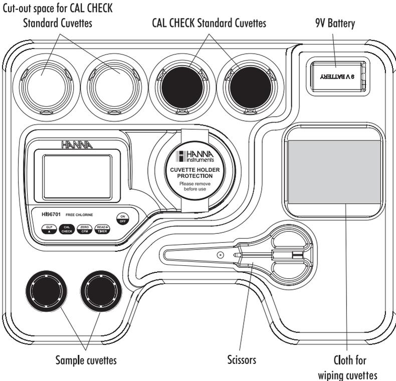
The **HI96701** is an auto diagnostic portable microprocessor meter that benefits from Hanna Instruments' years of experience as a manufacturer of analytical instruments. It has the advanced optical system based on a special tungsten lamp and a narrow band interference filter that allows most accurate and repeatable readings. All instruments are factory calibrated and the electronic and optical design minimizes the need of frequent calibration.
