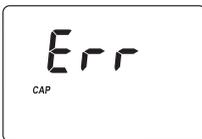
**Cap error:** Appears when external light enters in the analysis cell. Assure that the cuvette cap is present.
