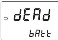
**Dead battery:** This indicates that the battery is dead and must be replaced. Once this indication is displayed, normal operation of the instrument will be interrupted. Change the battery and restart the meter.
