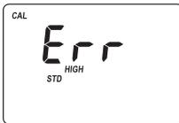
**Standard High:** The standard reading is higher than expected.
