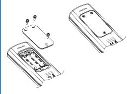
Replace the three 1.5V AAA alkaline batteries located in the battery compartment, observing the indicated polarity.
