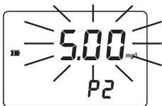
**Over Range:** A flashing value of the maximum concentration indicates an over range condition. The concentration of the sample is beyond the programmed range: dilute the sample and re-run the test.
