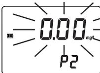
**Under range:** A blinking "0.00" indicates that the sample absorbs less light than the zero reference. Check the procedure and make sure you use the same cuvette for reference (zero) and measurement.
