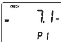
The reading should be within specifications as reported in the **CAL Check™** Standard Certificate. If the value is found out of the specifications, please check that the cuvettes are free of fingerprints, oil or dirt and repeat validation. If results are still found out of specifications, then recalibrate the instrument.
