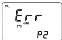
**Standard High:** The standard reading is higher than expected.
