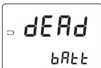
**Dead battery:** This indicates that the battery is dead and must be replaced. Once this indication is displayed, normal operation of the instrument will be interrupted. Change the battery and restart the meter.
