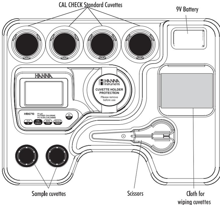
The **HI96710** is an auto diagnostic portable microprocessor meter that benefits from Hanna Instruments' years of experience as a manufacturer of analytical instruments. It has the advanced optical system based on a special tungsten lamp and a narrow band interference filter that allows most accurate and repeatable readings. All instruments are factory calibrated and the electronic and optical design minimizes the need of frequent calibration.
