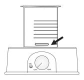
Pour the liquids to be mixed into the beaker. Do not fill the brim and leave sufficient space to prevent spillage during stirring.
