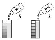
• Fill the color comparator cube with water sample to the 5 ml mark
