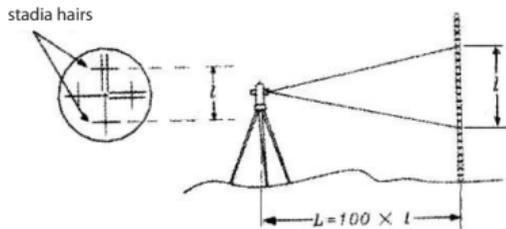
b. Level instrument. By viewing through the telescope, make sure the reading “ ” between two stadia lines.
