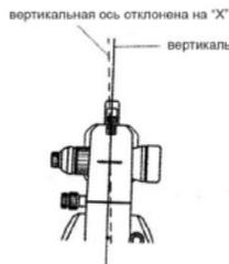
DigiTeo-2 has a vertical axis incline compensate. It can self-motion compensate the incline angle. When the incline sensor is switch on, the instrument can display the vertical axis incline angle. We can adjust the instrument level exactly by hand through the data. When it incline over the compensate arrange, the instrument display “TILT”. We must level the instrument.
