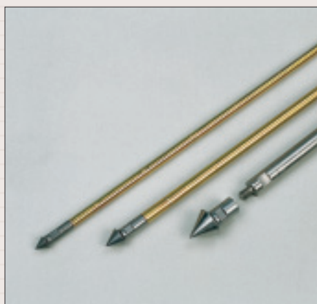
Cones and probing rods
