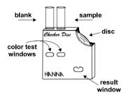
• Add to the other vial 1 packet of HI 3834-0 reagent. Replace the cap and shake to mix.
