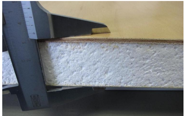
Example sandwich: aluminum - insulation - plywood
