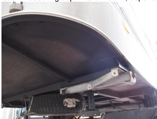
Caravan floor: massive flake board, little protected
