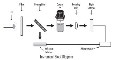
The internal reference system (reference detector) of the H197771 photometer compensates for any drifts due to power fluctuations or ambient temperature changes, providing a stable source of light for your blank (zero) measurement and sample measurement.
