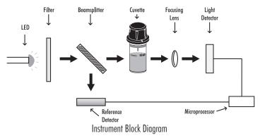
The internal reference system (reference detector) of the H197711 photometer compensates for any drifts due to power fluctuations or ambient temperature changes, providing a stable source of light for your blank (zero) measurement and sample measurement.
