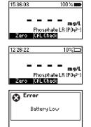
To conserve battery, the meter will turn off automatically after 15 minutes of inactivity. If a zero reading has been done but not a read, auto-off time is increased to 30 minutes.
