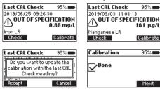
"OUT OF SPECIFICATION": A user calibration is not allowed, the measured value is outside of the tolerance window. Check the certified value, expiration date and clean the outside of the cuvette. Repeat the CAL Check procedure. If this error continues contact your nearest Hanna Instruments Customer Service Center.
