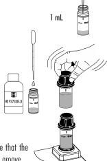
Press the Zero key. The display will show "-0.0-" when the meter is zeroed and ready for measurement.
