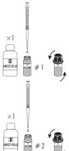
Add 1 drop of HI93719D-0 Magnesium Hardness Reagent D to the second cuvette (#2). Replace the plastic stopper and the cap. Invert several times to mix the solution. This is the sample.
