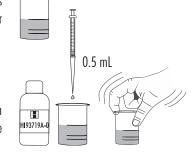
Add 0.5 mL of HI93719A-0 Magnesium Hardness Reagent A. Swirl to mix the solution.
