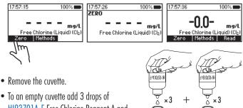
To an empty cuvetle add 3 drops of HI93701A-F Free Chlorine Reagent A and 3 drops of HI93701B-F Free Chlorine Reagent B.
