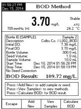
Note: No Seed correction is made in these calculations at this step. This may be made manually by subtracting the seed concentration from the samples, or made automatically with the meter (see SEED CORRECTION section).
