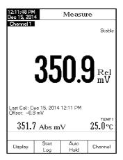
For greater accuracy, it is recommended to calibrate the ISE sensors frequently. The instrument should be recalibrated when "ISE x Calibration Expired" (the "x" represents channel "1" or channel "2") message appears on the LCD, in the Reminder messages area.
