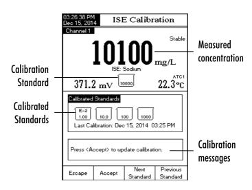
The group of calibration standards is set under ISE Setup  $\rightarrow$  Calibration. Select standards that are in the measurement range of the samples.
