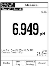
**Outside Cal Range** warns the user if the current reading is out of the calibrated area. The calibrated area is that part of the pH range in which the calibration point ensures an accurate reading. If the reading is taken out of the calibration area, the "**Outside Cal**
