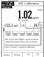
Press [Remove] to delete the selected calibrated point and then press [Accept] to update calibration with the new standard solution.
