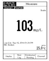
The measured concentration value will be displayed on the LCD. Press AutoHold" indicator will blink on the LCD until the stability criterion is reached. The concentration value will be frozen on the LCD, along with "AutoHold" indicator.
