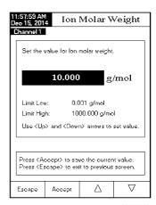
A pop-up menu will be displayed on the LCD, in which the slope value can be set using  $\triangle$  or  $\nabla$ . Press Accept to save the modified value or press Escape to return to the previous menu.
