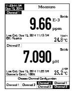
For each measurement mode (pH, mV, Rel mV or ISE) the following display configurations are available: Basic, Good Laboratory Practice (GLP) (pH, ISE only), Graph and Log History.
