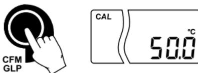
Submerge the temperature probe (or EC probe) in the second vessel as near as possible to the calibrated thermometer. Allow a few seconds for the probe to stabilize.
