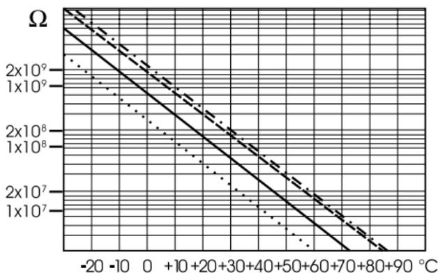
Since the resistance of the pH electrode is in the range of 50–200 Mohm, the current across the membrane is in the pico Ampere range. Large currents can disturb the calibration of the electrode for many hours. For these reasons high humidity environments, short circuits and static discharges are detrimental to a stable pH reading.
