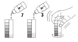
• Remove the cap from the plastic vessel. Rinse the plastic vessel and fill to the 25 mL mark with water sample.
