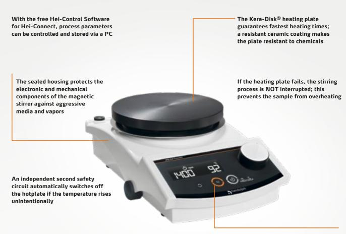
Damage to the device is impossible even at the highest temperatures – all models are equipped with a fire-resistant die-cast housing The device is switched off completely in the event of a short circuit, broken sensor of the temperature sensor and in the event of a processor fault
