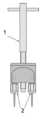
Insert needles into the needle-holder (2) and tighten with a flat wrench (wrench size 12 mm). Its essential to verify that the needles are tightened well enough before punching the electrode into materials.
