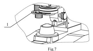
Place ground glass 1 on the filter seat, turn the filter seat in observation position when observe the specimen image with 4X or 10X objective.
