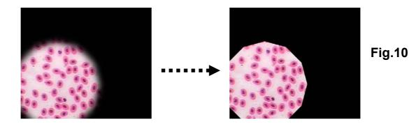
8. If the image of field diaphragm is not centered in the field of view, proceed to its centering acting on the appropriate side condenser centering screws (E) until the image of field diaphragm is brought into the center of the field of view, <u>like in fig.11</u>.
