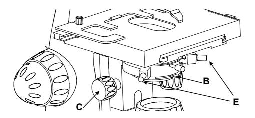
7. Now close the field diaphragm (A) of the illuminator about half of its total aperture and, through the appropriate side knob (C), regulate the height of condenser until the image of the contour (or part of it) of the field diaphragm with its sheets can be observed clearly, <u>like in fig.10</u>.
